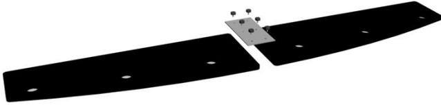
**Steps 2-4.** Flip canopy over and attach left and right upper column sections using 2 **short** knobs per column. Install gusset caps. Attach header grippers.
