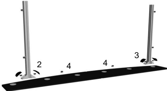
**Steps 5,6.** Attach left and right lower columns to feet using 2 **short** knobs per column. Install gusset caps.
