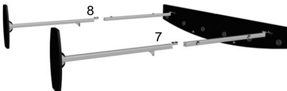
**Step 9.** Lift canopy into position. Attach graphic panels using 2 **short** nylon tipped knobs per panel.
